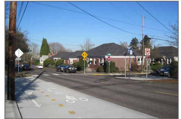
A grade separated cycle track can help bicyclists comfortably transition through a jog in a Neighborhood Bikeway
