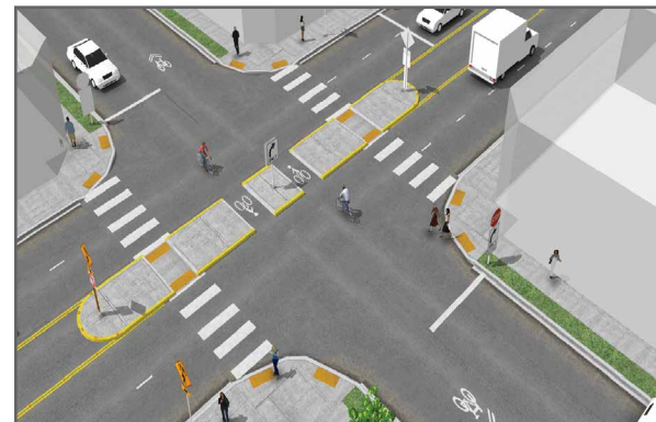
The preferred design for median diverters includes separate median refuges for bicyclists and pedestrians to minimize conflict between users
