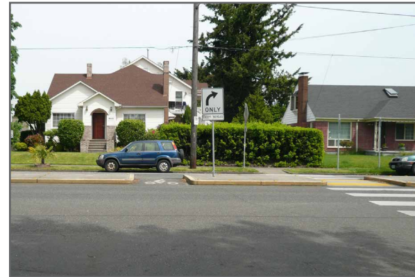
Median diverters assist with volume management on Neighborhood Bikeways by directing motor vehicles to use alternate routes
