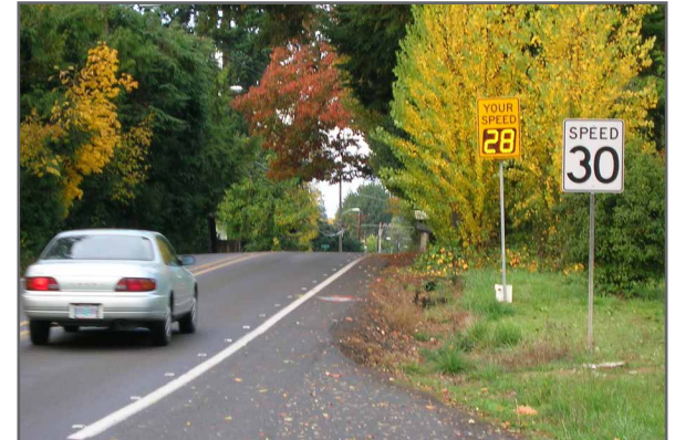
Speed reader boards use radar to alert drivers of current speed and encourage them to slow down. This is a permanent installation.
