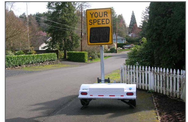
Speed reader boards can also be used on moveable trailers or platforms so that they can be moved to various locations for shorter durations.
