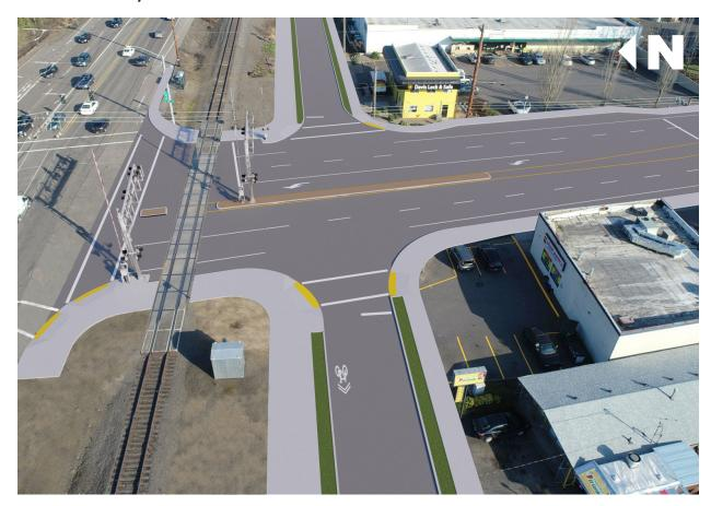
The short distance between TV Highway and Shaw Street at SW 170th Avenue makes a half signal at this location very unlikely. The crossing at TV Highway could be improved to simplify the crossing as shown in the figure above. This requires removing the pork chop island for the eastbound right-turn and relocating the signal and utilities located on the island to the corner.
