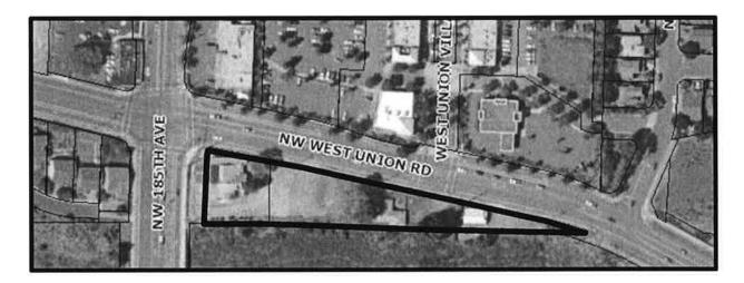
D. The applicant proposes two points of access: 1) a westerly driveway designed as a restricted right-in only access, and 2) an easterly driveway aligned with the existing signalized intersection of the West Union Village entrance (the signalization is currently only for 3 legs of the intersection and the applicant will be required complete the fourth leg of the intersection).
