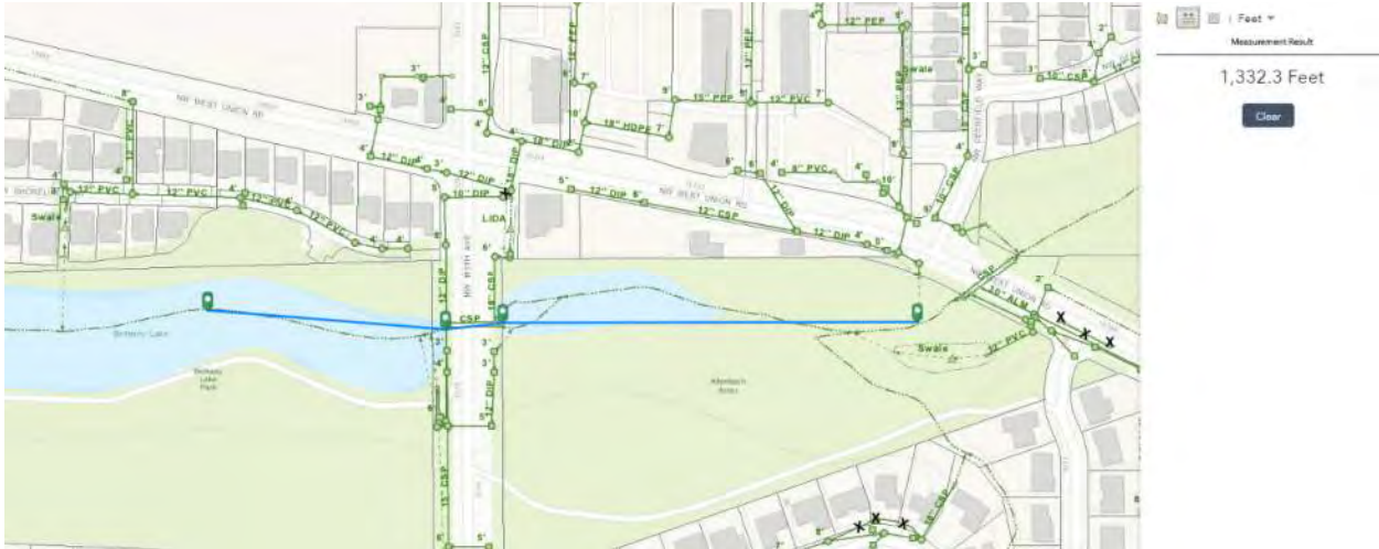
CWS Sanitary & Storm Sewer Map – Extent of Downstream Analysis
